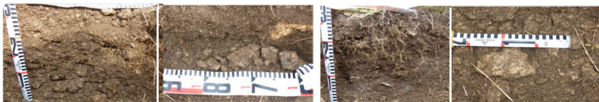
Figure 9: Cross sections with about 20-cm-depth-roots in 30 cm layer and stones (left: 21-year-past in Process 1 showing 6~3 cm stones, right: 18-year-past in Process 2 showing 9~3 cm stones)
