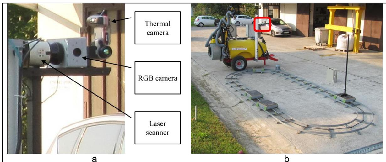
Figure 3 - Selective sprayer. (a) sensors array, (b) overall sprayer with rail (red square, sprayer sensors)
