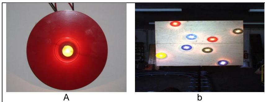
Figure 1 - ACP's. (a) single target with a 10W light bulb in the middle, (b) flat plate with 8 CP targets
