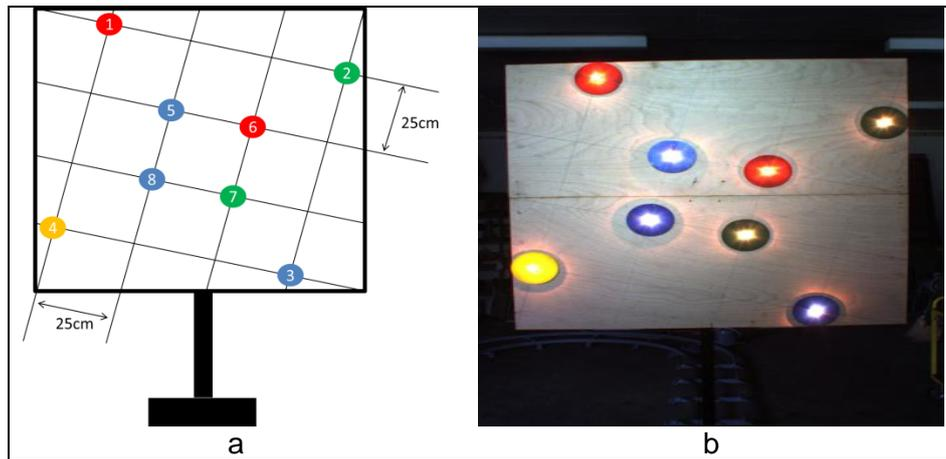
Figure 2 - ACP's arrangement (a) and sample RGB image of ACP's mounted on a plate.
