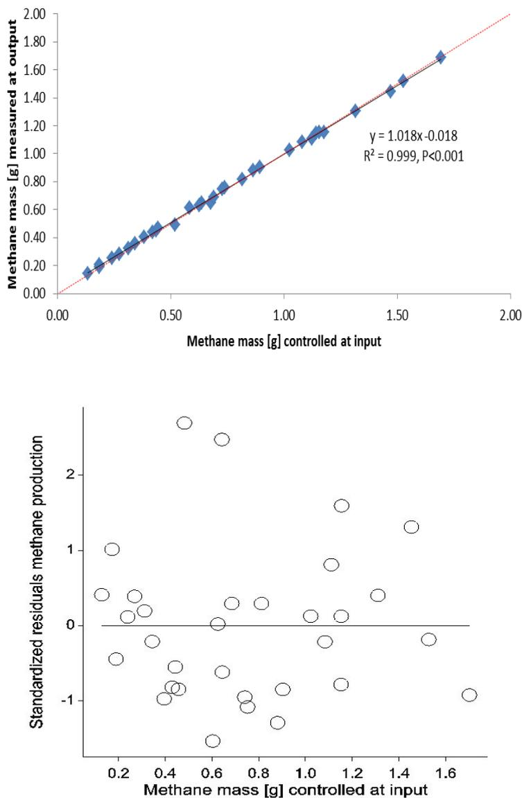
Figure 3. Methane mass [g] controlled at input versus measured at output (above) and standardized residuals (below) versus methane production [g] during each 8 minutes experiment; the dotted line (above) represents the line of equivalence.
