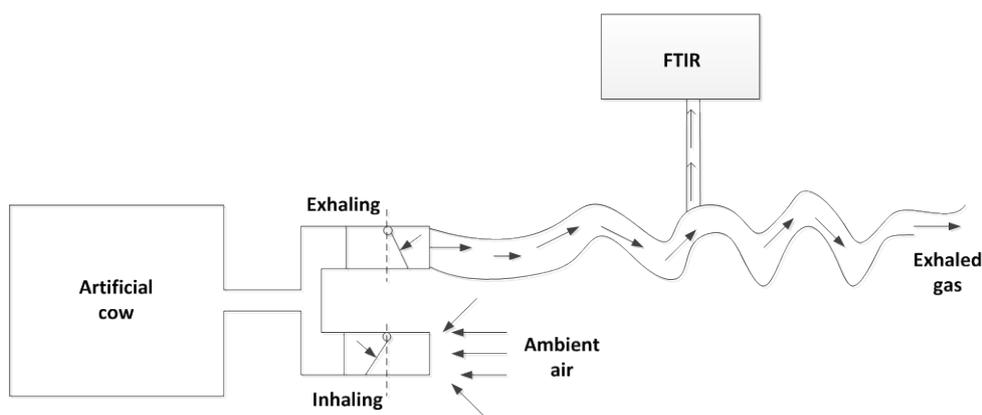
Figure 2. Schematic of the experiment setup to evaluate methane mass balance of the artificial reference cow.
