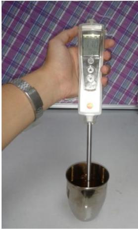
Figure 2: TPC measurement using (Testo 270, InstruMartInc, Germany).
