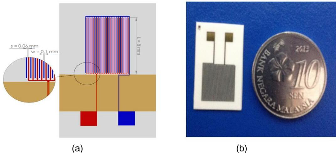
Figure 1: (a) A top-view illustration of impedance sensor probe, (b) A photograph of prototype device next to a Malaysian coin.
