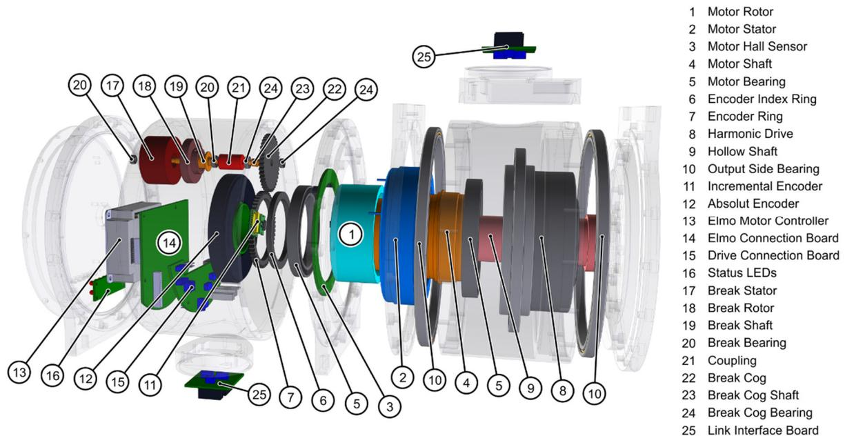
Figure 3: Exploded view of a the big drive unit
