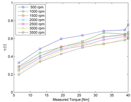
Figure 7: Efficiency measurement for different speeds
