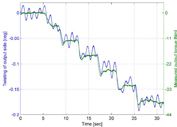
Figure 6: Comparison between measured output torque and twisting of the drive unit (measured with test bench encoder)
