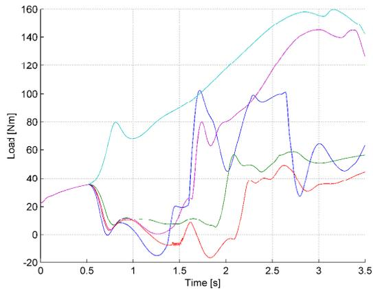
Figure 1: Dynamics simulation of joint 3 for five different harvesting motions
