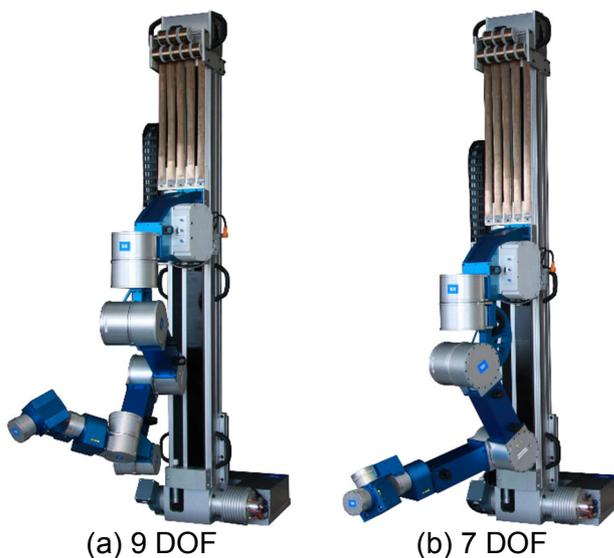
Figure 8: Manipulator prototype generation 2 (2014)
