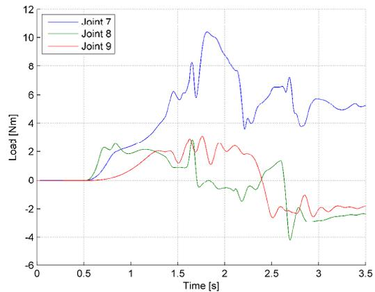
Figure 2: Dynamics simulation of joint 7, 8 and 9 for a harvesting motion
