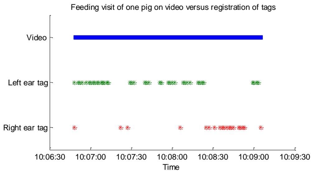
Figure 3: Feeding visit of one pig on video with the corresponding RFID registrations of both transponders.
