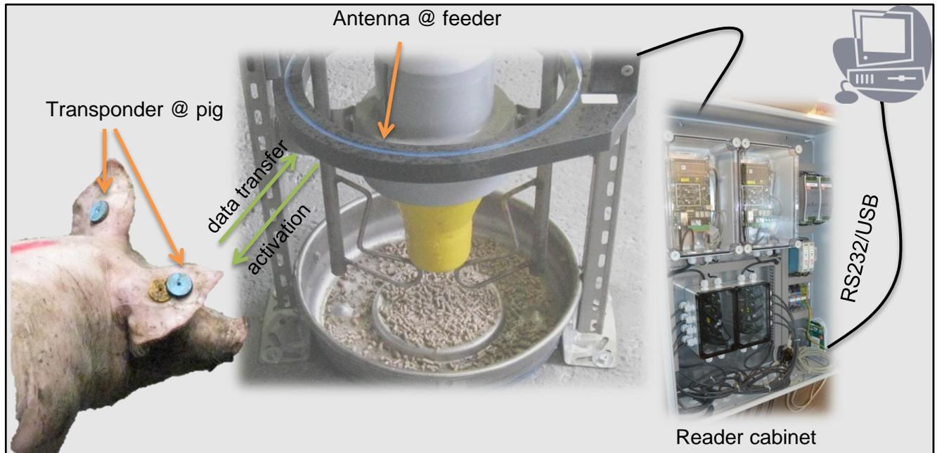
Figure 1: Overview of the different components of the passive High Frequency RFID system.
