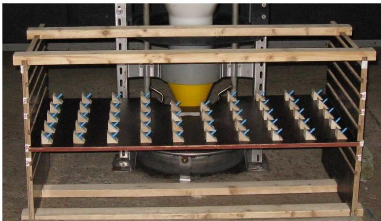
Figure 2: Test set-up for the offline validation, using this board transponders could be placed under an angle of 45° with the horizontal.
