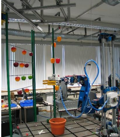
Figure 5 Laboratory testbed at TUM for harvesting sweet-pepper and apples. The fruits are hinged with magnets on stems, which hang from the top and can be adjusted in the x - y plane.
