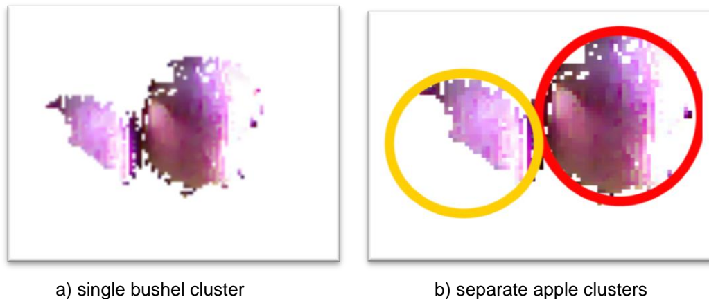
Figure 4: Illustration of the post-processing algorithm for separating a single bushel cluster identified by the Euclidean clustering algorithm into separate apple clusters (circles with different color)
