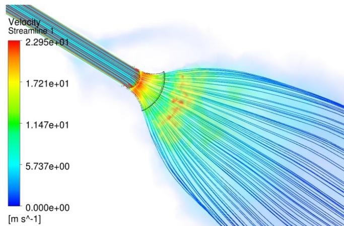
Figure 4: Streamlines and velocities for straight air supply pipe
