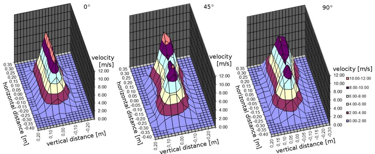
Figure 6: Velocity profiles for different joint angles measured 0.5 m away from the exit
