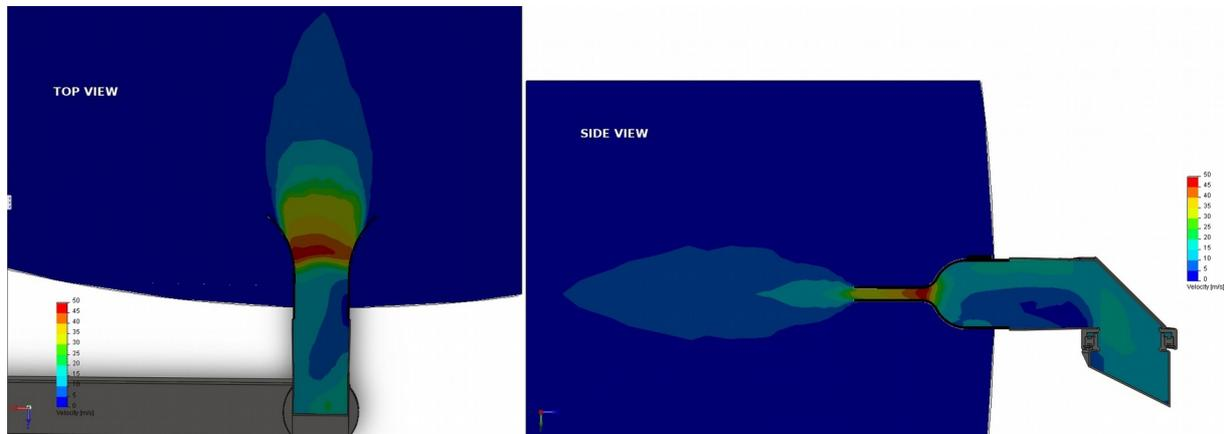
Figure 5: Air velocities for the prototype spraying arm with a joint angle of 90° (top and side view)
