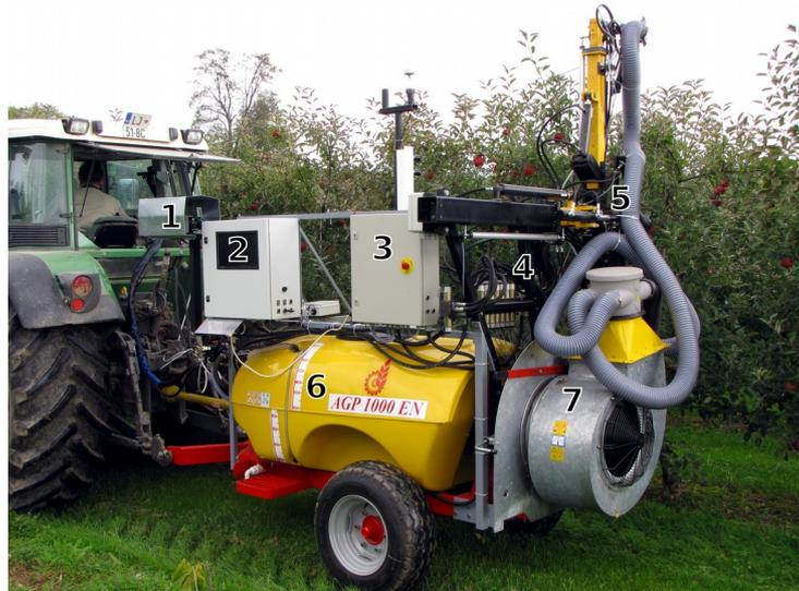
Figure 2: Orchard sprayer with LIDAR (1), computer (2), electronics (3), electromagnet valves (4), spraying arms and air ducts (5), tank (6) and radial fan (7)
