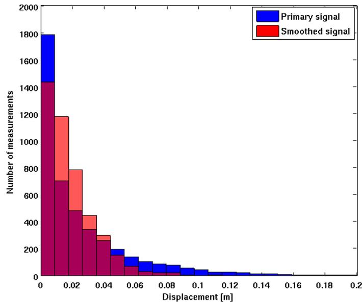
Figure 5: Comparison of arm displacements before and after smoothing
