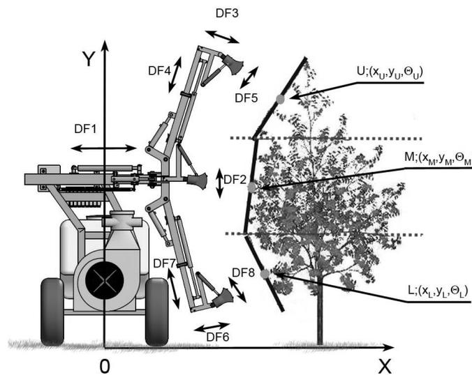
Figure 1: Canopy adapted spraying based on LIDAR data
