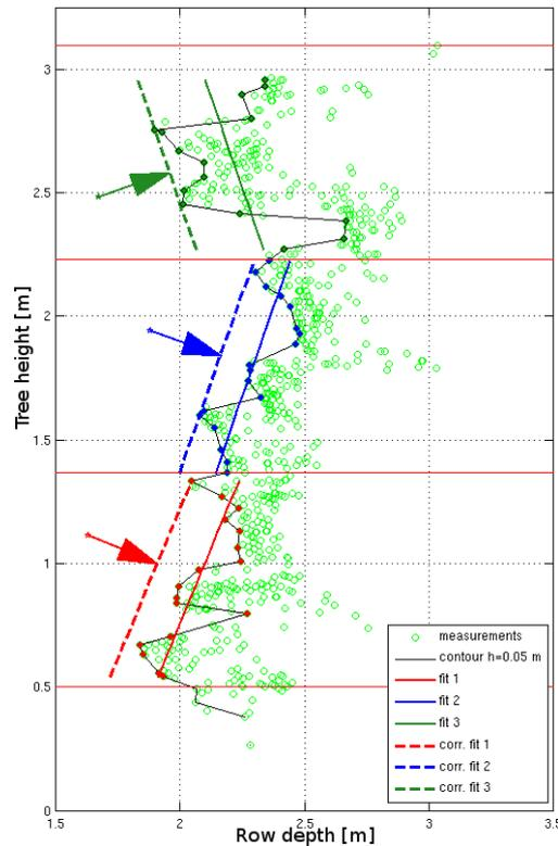
Figure 3: Positioning of spraying arms based on LIDAR data
