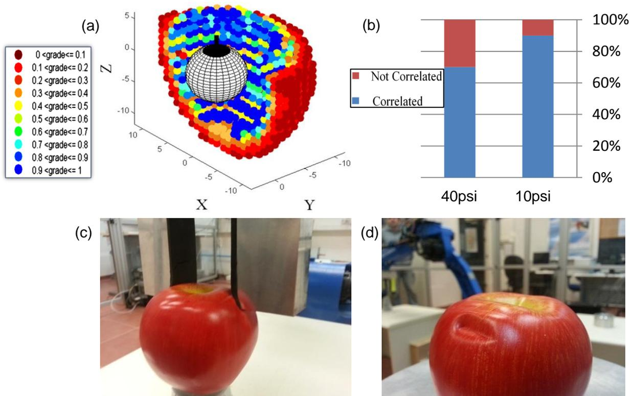
**Figure 2:** (a)  $Q_{FS}$  graspability map, values range from 0...1, where 0 indicates bad grasp and 1 good grasp. Only half the map is plotted for presentation clarity. (b) Correlation between  $Q_{PHYS}$  and  $Q_{FS}$  (c) Execution of a problematic grasp (d) Damage caused by the grasp.
