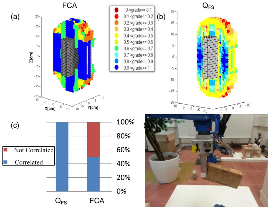
**Figure 3:** (a) FCA graspability map. (b)  $Q_{FS}$  graspability map, values (both a and b) range from 0...1, where 0 indicates bad grasp and 1 good grasp (c) Grade comparison between  $Q_{PHYS}$  and  $Q_{FS}$  (d) Grasp Demonstration.
