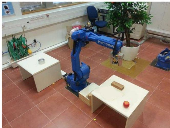
**Figure 1:** The physical environment, the robot, the gripper and the objects (plastic apple, cube).
