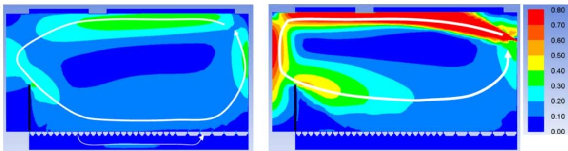
Figure 4. CFD prediction of air flow pattern and velocity ( $m s^{-1}$ ) distribution in symmetry plane of a pig pen at outdoor temperature of 10 °C without PPAE: (a), Diffuse ceiling air inlet; (b), Diffuse wall jet inlet (Bjerg & Zhang, 2013).
