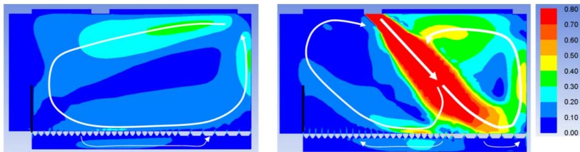
Figure 3. CFD prediction of air flow pattern and velocity ( $m s^{-1}$ ) distribution in symmetry plane of a pig pen at outdoor temperature of 20 °C without PPAE. (a), Diffuse ceiling air inlet; (b), Diffuse ceiling air inlet in combination with ceiling air jet inlet (Bjerg & Zhang, 2013).
