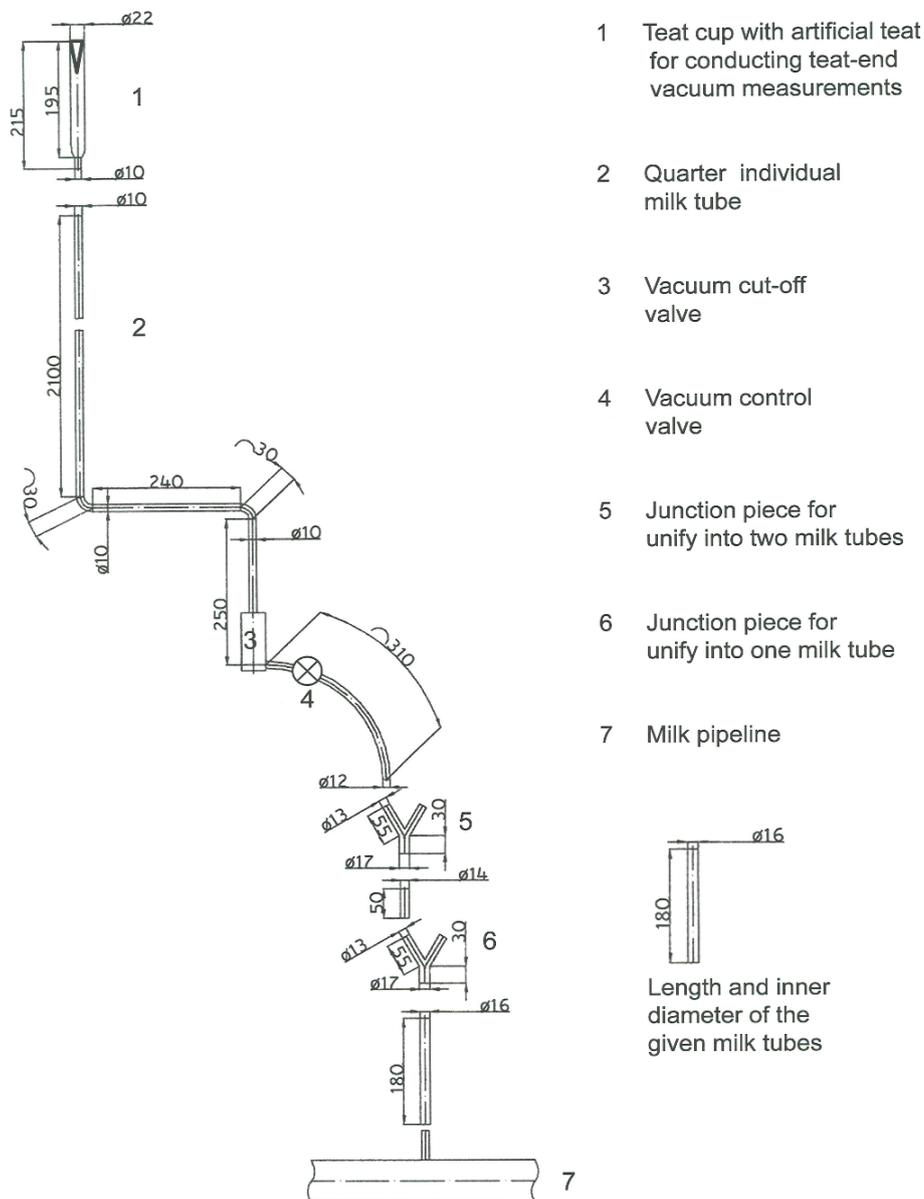
Figure 1: Schematic drawing of the test set-up: The duct system of the Multilactor® milking system with inserted vacuum control valve (VCV) (Ströbel et al., 2011).
