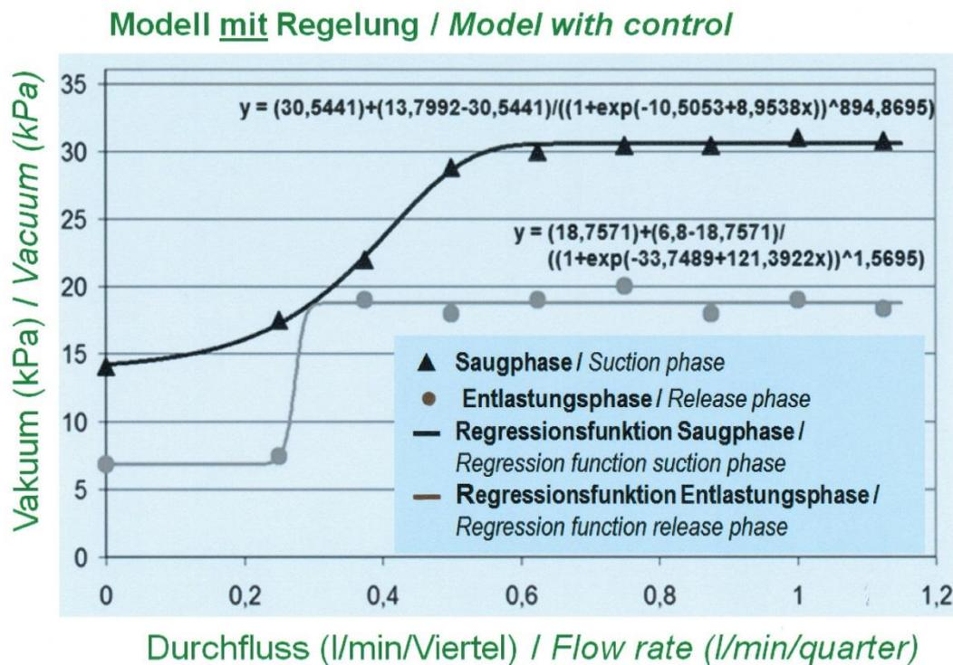
Figure 2: Effect of the vacuum control unit on the teat-end vacuum depending on the milk flow rate (Ströbel et al., 2011).
