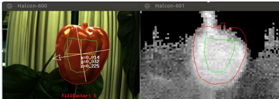
Figure 5: Images of the cameras on the end-effector. Registered colour image (left), registered ToF distance image (right)
