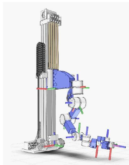
Figure 2: Rendering of the 9 DoF robotic manipulator
