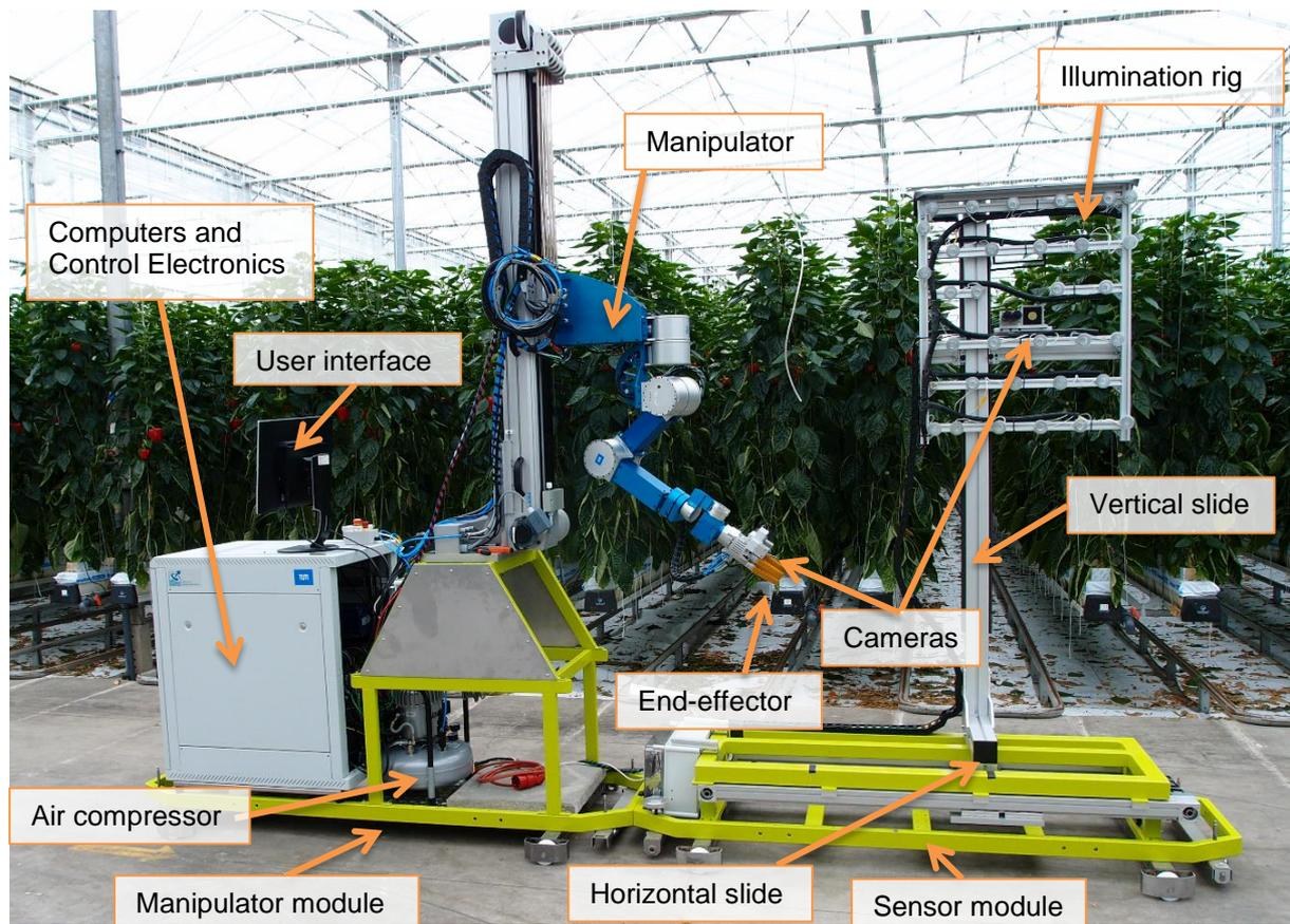
Figure 1: Integrated robotic system for harvesting sweet-pepper fruit.
