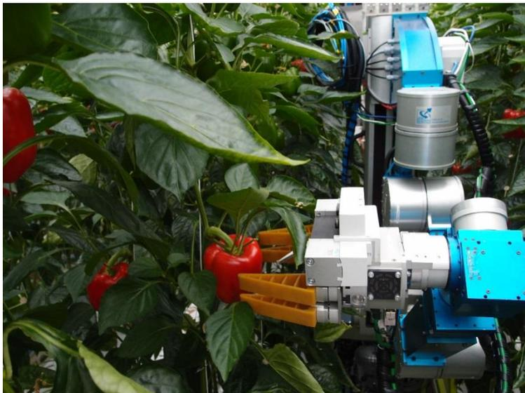
Figure 6: Harvesting robot in the greenhouse
